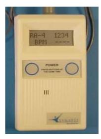
The stimulator can only be programmed by a clinician using a separate programming station. The only settings on the stimulator are two "power" buttons which must both be pushed simultaneously to either "turn on" or "turn off" the stimulator (a safety feature to guard against inadvertent inactivation).
