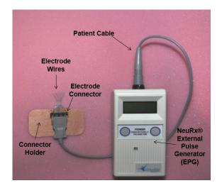
The external components of the NeuRx<sup>®</sup> DPS include the External Pulse Generator (EPG) or stimulator, the patient cable, and the implanted diaphragmatic electrode wires which are connected to the patient cable via the electrode connector or "block". The electrode connector is attached to the chest wall using an adhesive connector holder.
