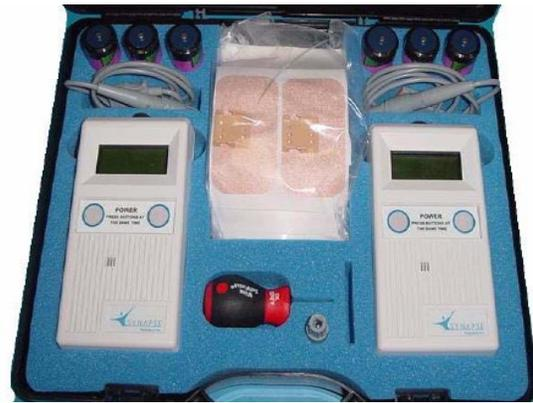
The DPS Patient Kit consists of a black plastic briefcase containing the backup stimulator, spare batteries, a screwdriver (to replace the battery in the stimulator), and spare connector holders. The spare stimulator should be available at all times should the stimulator in use develop problems. The two stimulators are typically programmed with the same settings and should be alternated to maintain the charge on the internal batteries
