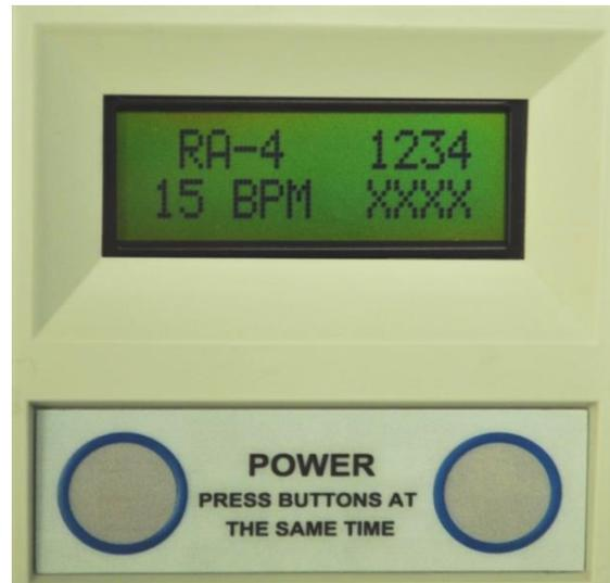
If ‘X’ appears below one or more output numbers, one or more electrode wires may be loose or broken, the patient cable may be broken or not connected properly, or the stimulator may be broken. The stimulator should be changed, and the patient’s surgeon notified.
